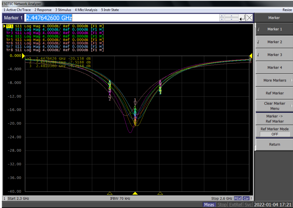
Figure 5.9. Antenna Return Loss for Outer Antenna (JL-2800 laminate)
